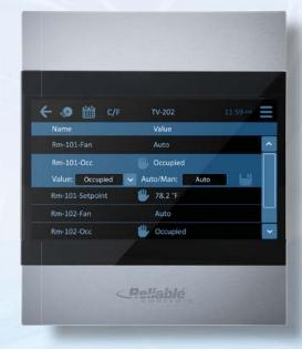
LISTview: allows ease of access for operators and end users to view and adjust critical parameters without having to enter the grow area.
